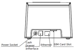
Figure 2-1 Printer Part Name Diagram
